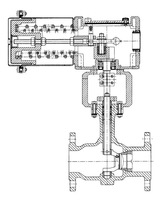
with rotary actuator BR99-1-NT BR99-2-NT / BR99-3-NT
