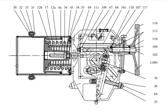
Pos. 55 Radial shaft seal Pos. 56 Circlip Pos. 57 Retaining ring Pos. 58 Needle bearing Pos. 63 Sealing plug Pos. 64 Cap nuts Pos. 65 Setscrew Pos.101 Flange Pos.102 Adjusting bolt Pos.107 Retaining ring
